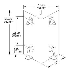
SSPAM-204-2P-HC VX 16.00 408mm CEILING A SUFFIX VX (For 3ISA& 204 units) 22.00 559mm VX length: 22.00 To Calculate: 559mm VX Length = Ceiling height minus SHOWER HEAD 44.00 1118mm HEIGHT Shower head height minus 5" (127mm) 3ISA (Ceo 7.00 178mm 8 1/4" (209mm) 204 19.00 483mm 1.75
